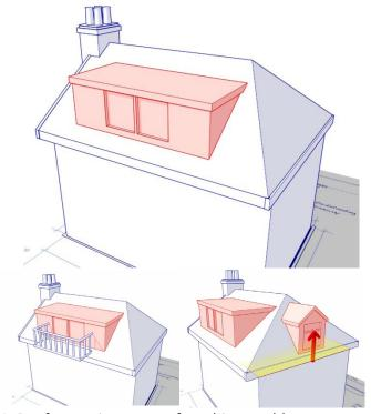
**8.** Roof extensions, apart from hip to gable ones, to be set back, as far as is practicable, at least 20cm from the original eaves. The 20cm distance is measured along the roof plane.
